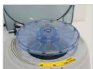
Microhematocrit rotor for 12 tubes
