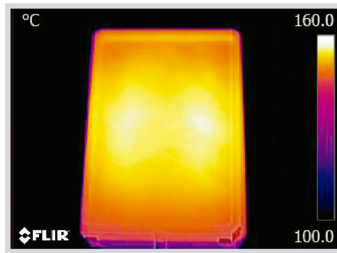
Figure 2. Thermal Image of a Competitive Hotplate
