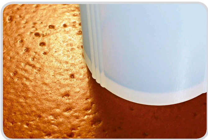
Figure 4. Competitive Hotplate Image Showing Deep Pores in the Surface
